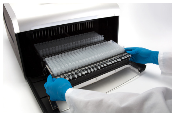
Figure 39. Placing the cartridges in the Deck Tray and pressing firmly to snap them in place.
