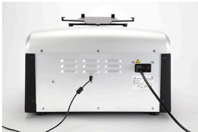
Figure 10. Connecting the Tablet PC to the back of the Maxwell® CSC 48 Instrument.
