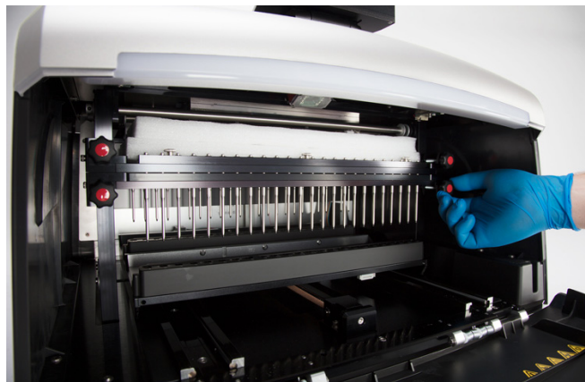
Figure 62. Placement of plastic stoppers. Move the magnet and plunger bars up, and secure the four shipping screws on both sides of the magnet and plunger bars.
