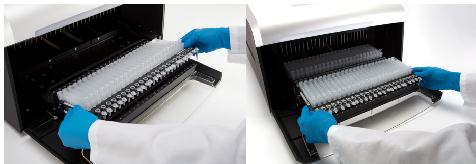
Figure 41. Placing the deck tray in the instrument.
