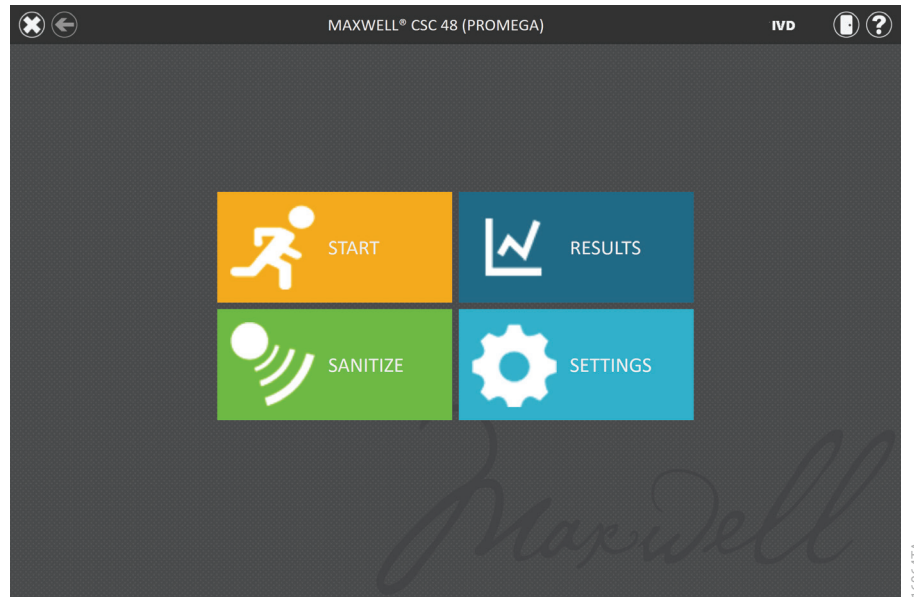
Figure 32. Maxwell® CSC 48 'Home' screen. Selecting the Start button begins the process of running an extraction method on the Maxwell® CSC 48 Instrument.
