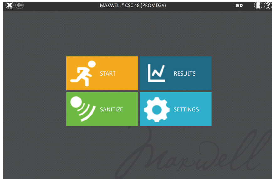
Figure 53. Maxwell® CSC 48 'Home' screen. Selecting Results opens the Maxwell® CSC 48 'Results' screen from which extraction reports from all method runs can be viewed.
