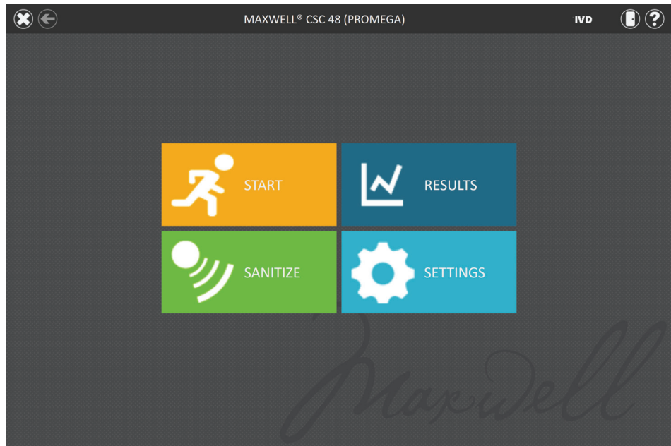
Figure 56. 'Home' screen. Selecting the Sanitize button begins the process for UV treatment of the Maxwell® CSC 48 Instrument.
