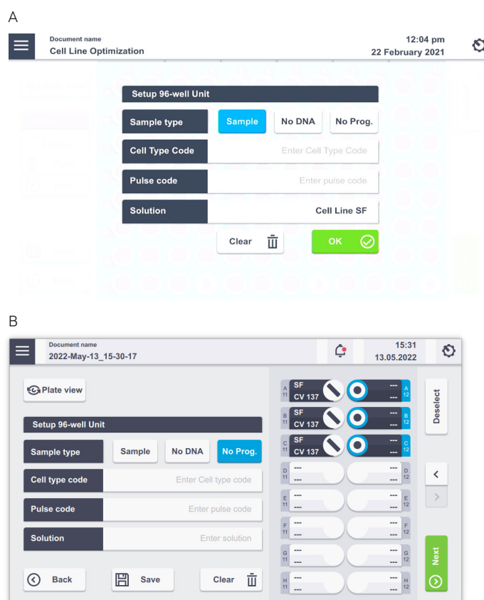
Figure 2.30 A: Experiment settings after well selection and tapping on “Edit” button in plate view (A) and Sample definition in strip view (B).
