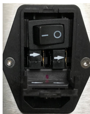
Figure 2.1: Opened fuse receptacles
