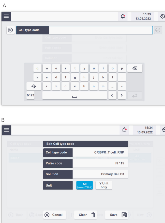
Figure 2.50: (A) Typing the name of the custom Cell Type Code. (B) Overview of conditions for custom Cell Type Code. Press “Save” to save the conditions, press “Clear” to start again.
