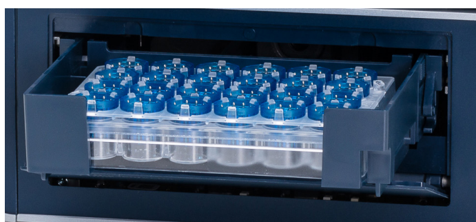
Figure 2.26: Loading of samples (Y Unit). Watch the orientation of the plate. (Well A1 is placed in the upper left position).
