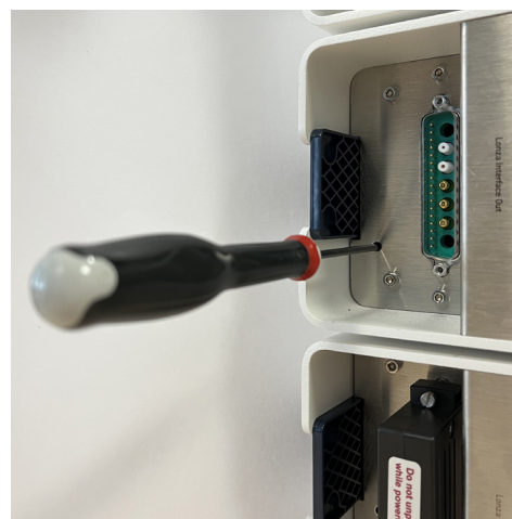
Figure 2.9: The position of hexagon screw driver during manual adjustment of 4D-Nucleofector® System to the transportation mode.
