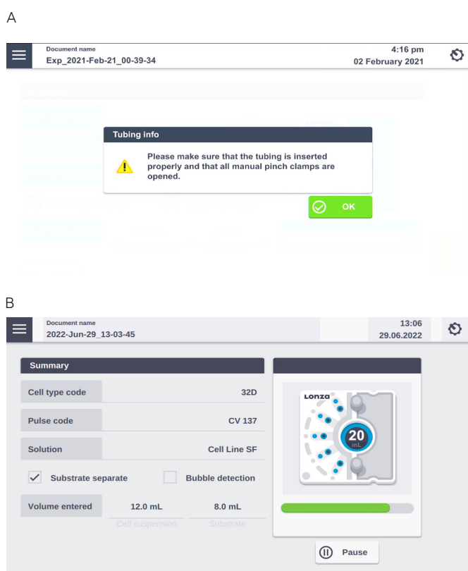
Figure 2.43: (A) Prompt before starting the actual experiment to check tubing and open clamps. (B) Progress of the experiment.
